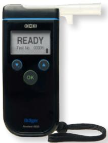
The Alcotest 6820 handheld breath alcohol detection device, manufactured by Dräger Safety, is a compact, robust, and easy to use device. It can be conveniently held in one hand, and intuitively operated with clear and concise menus. The display is easily read in any lighting condition.
